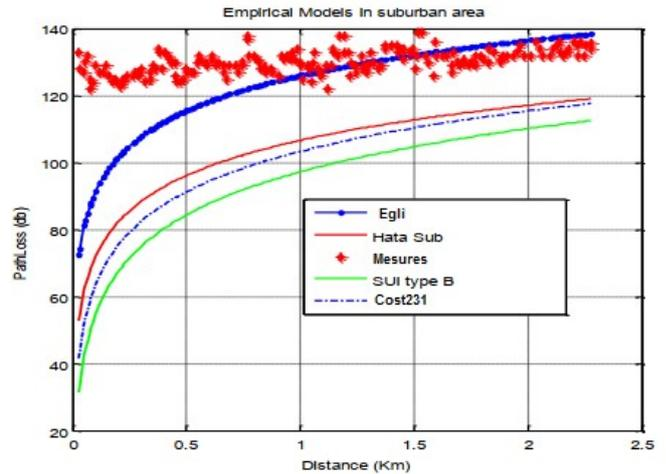
Fig 1. Comparison between predicted and measured path loss for BTS1
