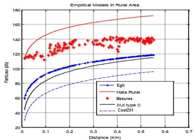
Fig 2. Comparison between Predicted and Measured Path Loss for BTS2
